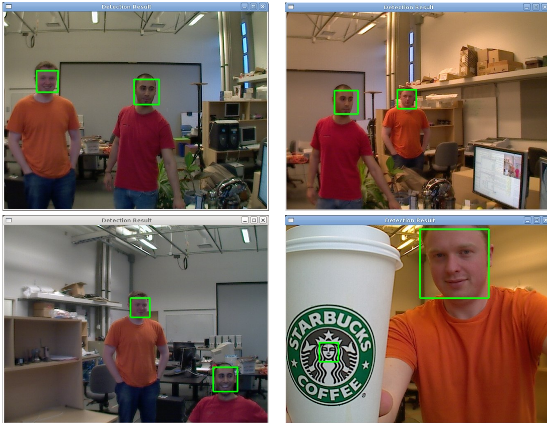
Fig. 6. Results of the face detection application running on a Hive system distributed across four drones, with one application in control which displays the result (shown).
